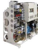
Electronically controlled pneumatic brake
