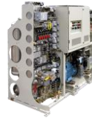
Electronically controlled pneumatic brake
